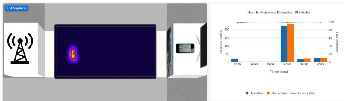
Figure 51. JCAS/ISAC demonstration: heatmap and hourly presence detection statistics
