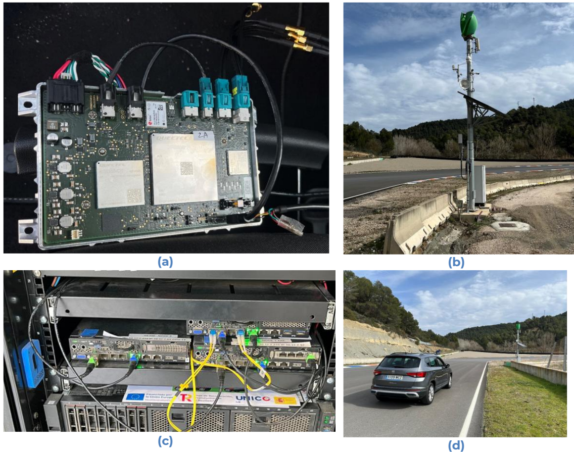
Figure 30:: Experimental setup at the Circuit Parcmotor Castelloli: (a) On-board unit used in the trials, (b) 6G SA gNB, (c) Edge servers in the control room, (d) Vehicle approaching the gNB.
