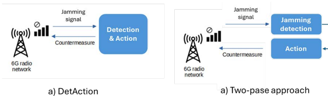
Figure 7: Anti-jamming system approaches.
